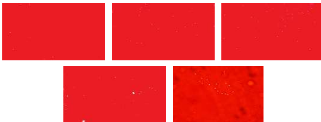
Figure 5. Photomicrographs for the revelation of the alpha particle tracks observed in five LR-115 detectors placed at the top of the rock samples
