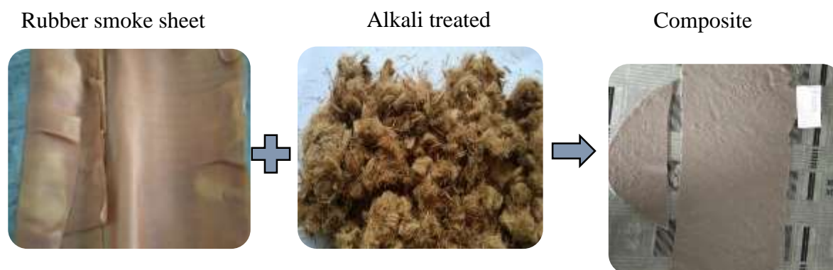
Figure 1. Preparation of alkali treated areca nut fiber-rubber composite for stopper
