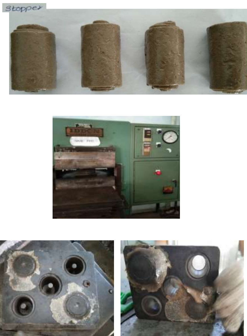
Figure 2. Making of alkali treated areca nut fiber-rubber stopper
